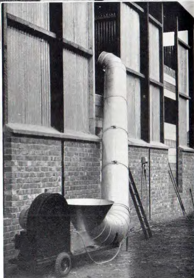
Right: Pneumatic conveyor for delivering cut grass to centre bay. The conveyor is mobile.
